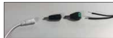
2 Conductor Wires running to basement 12V Power Transformer
